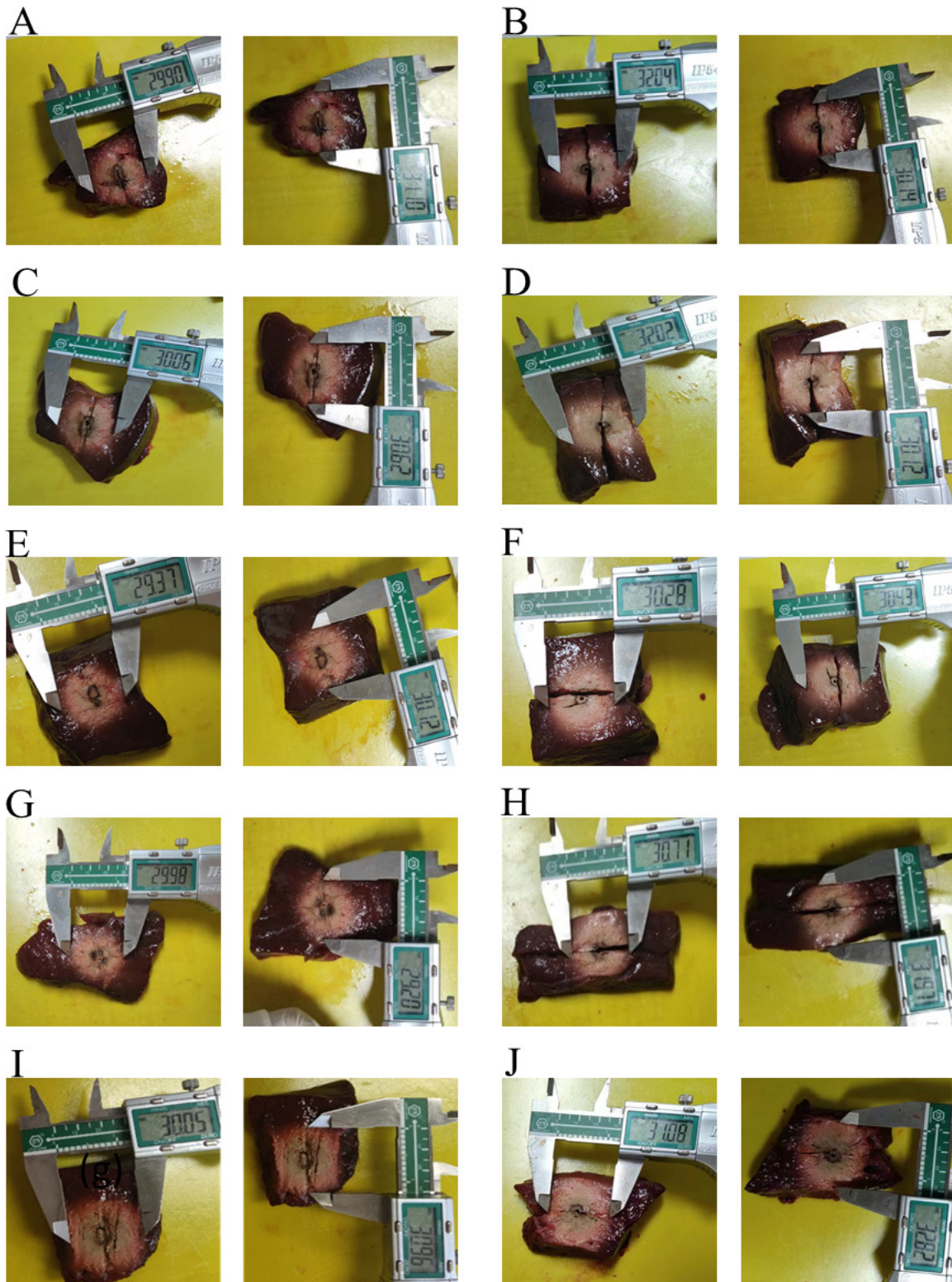
Figure 7. Experimental plots of five groups of boundary temperature-controlled ex vivo bovine livers. (A) The axial plane of the first ablation region; (B) The transverse plane of the first ablation area; (C) The axial plane of the second ablation area; (D) The transverse plane of the second ablation area; (E) The axial plane of the third ablation region; (F) The transverse plane of the third ablation area; (G) The axial plane of the fourth ablation area; (H) The transverse plane of the fourth ablation area; (I) The axial plane of the fifth ablation region; (J) The transverse plane of the fifth ablation area.
